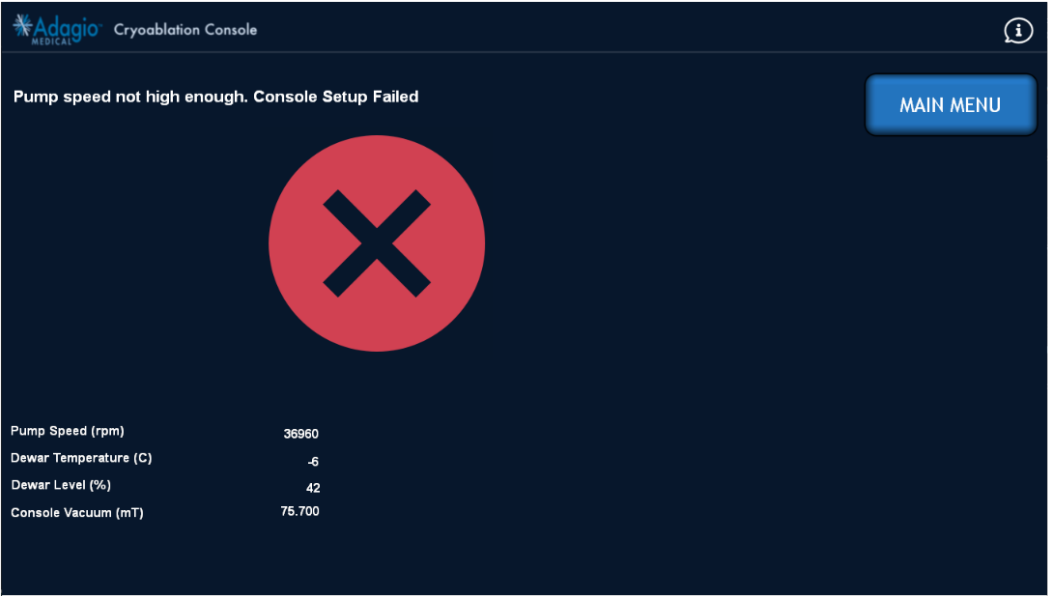
Figure 74 – Prepare Console Test Failed (Not Enough Pump Speed) Screen Image
