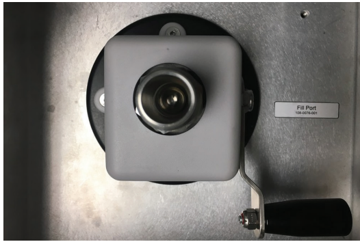
Fill Valve Closed
