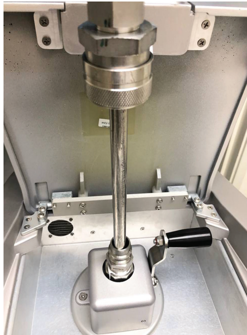
Figure 24 – Pulling Back On The Fill Tube Collar To Lock Into The Fill Port
