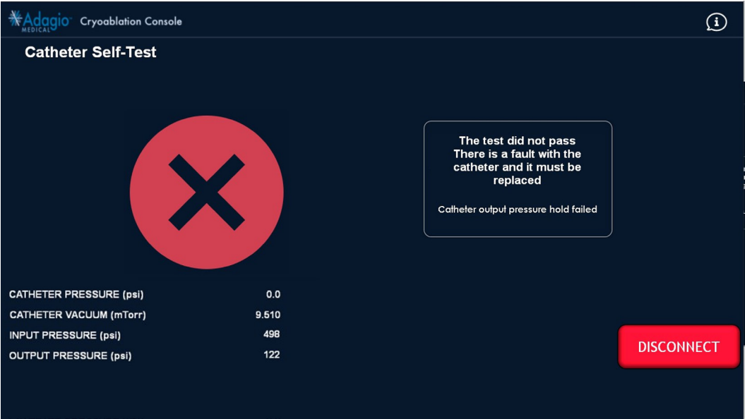
Figure 42 – Catheter Self-Test Fail (Output Pressure Hold Failed) Screen Image
