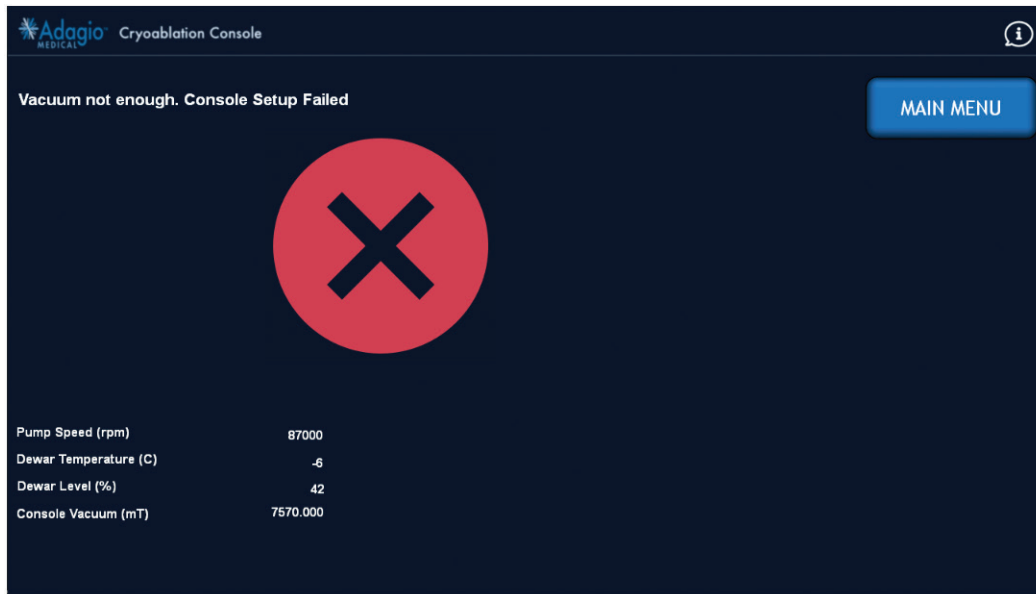
Figure 18 – Prepare Console Test Failed (Not Enough Vacuum) Screen Image
