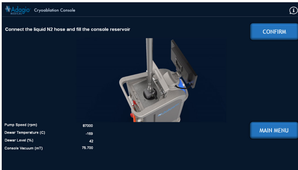
Figure 76 – Connect The Liquid N2 Hose To The Console And Fill Its Internal Reservoir Screen Image
