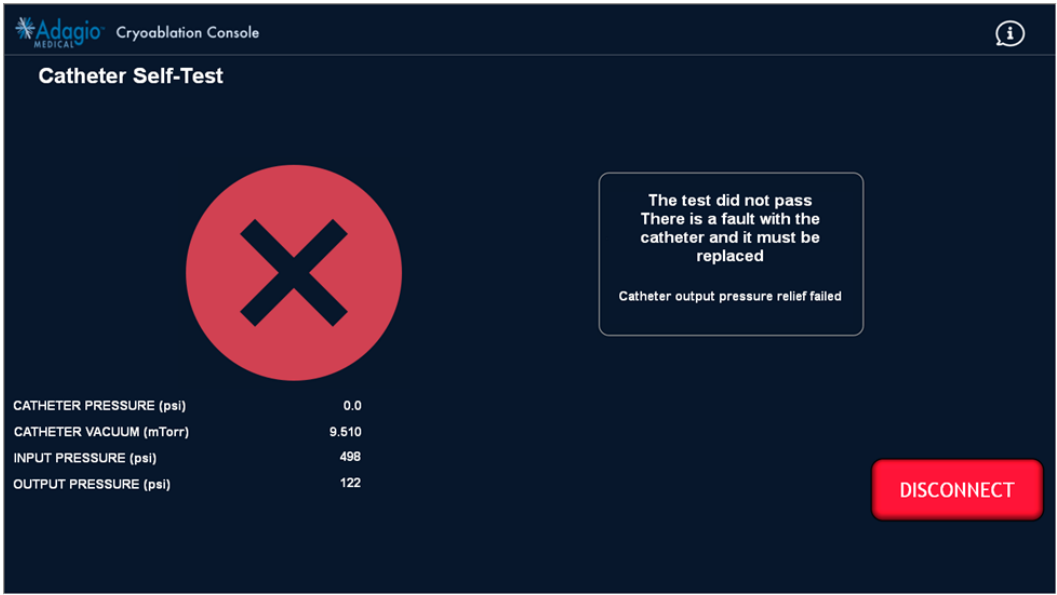
Figure 41 – Catheter Self-Test Fail (Output Pressure Relief Failed) Screen Image
