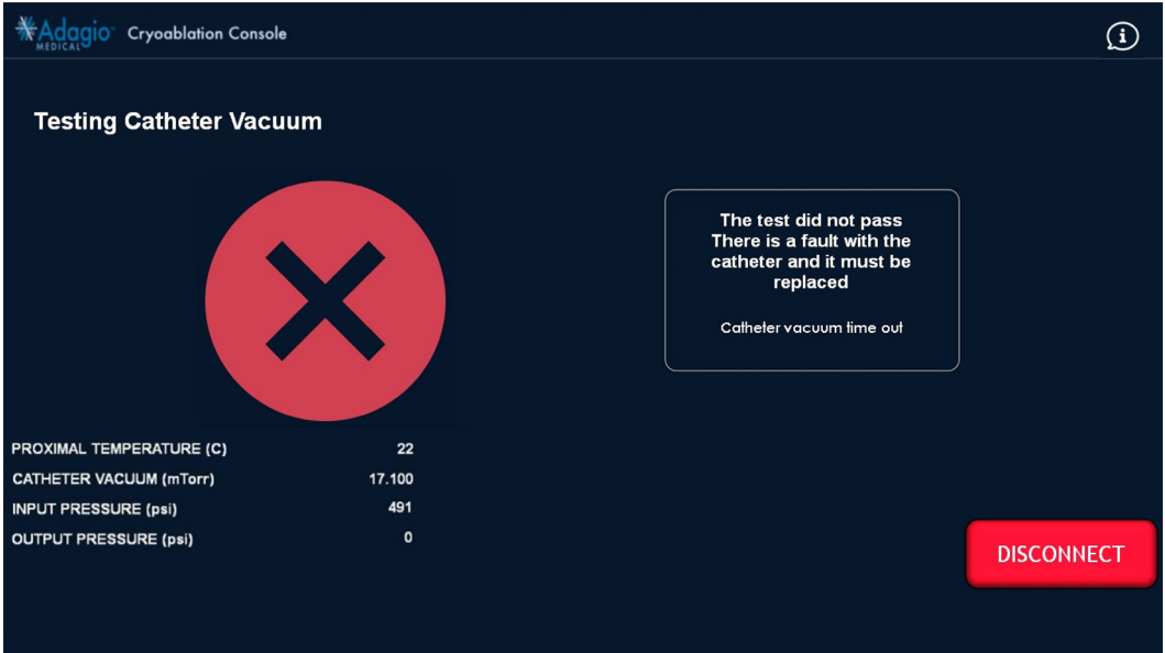
Figure 86 – Catheter Vacuum Test Fail (vacuum and output pressure time out) Screen Image
