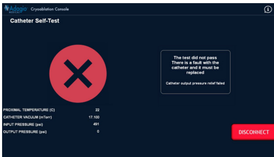
Figure 91 – Catheter Self-Test Fail (Output Pressure Relief Failed) Screen Image
