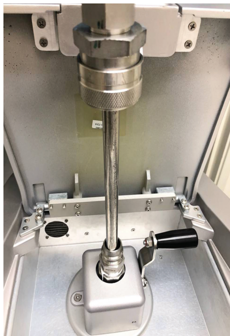
Figure 79 – Pulling Back On The Fill Tube Collar To Lock Into The Fill Port
