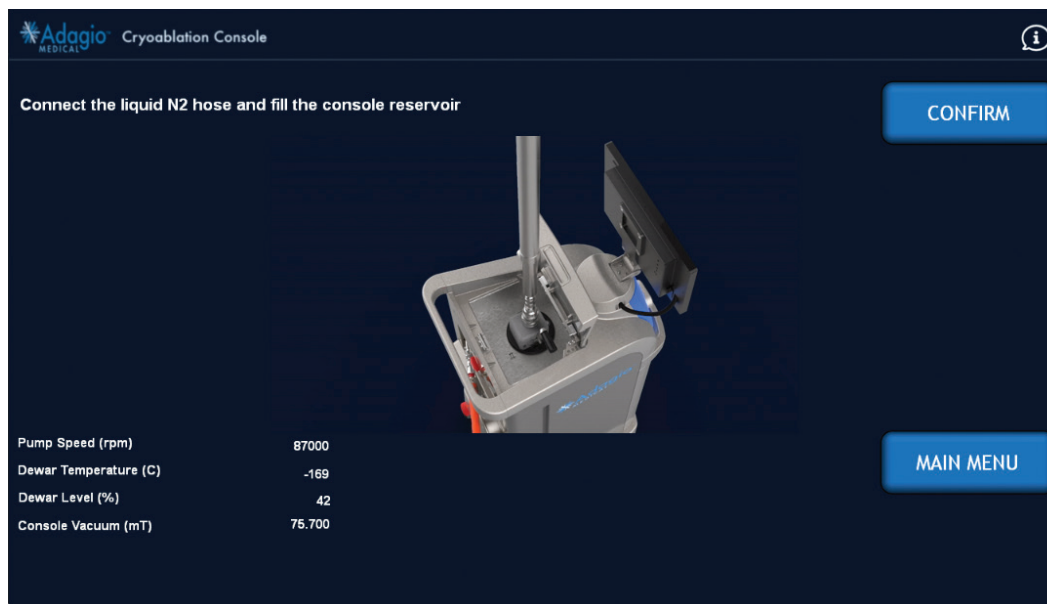
Figure 21 – Connect The Liquid N2 Hose To The Console And Fill Its Internal Reservoir Screen Image
